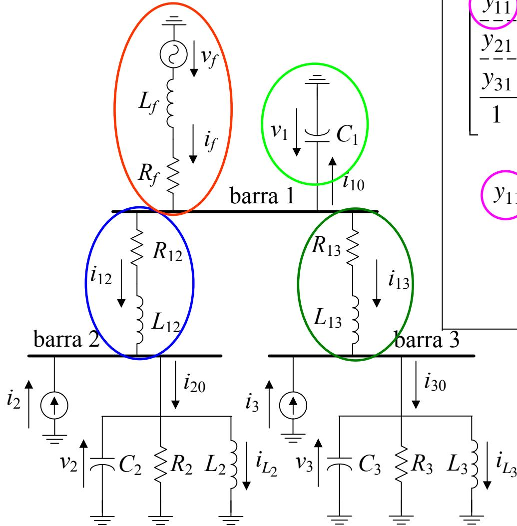
$$\begin{bmatrix} y_{11} & y_{12} & y_{13} & -1 \\ y_{21} & y_{22} & 0 & 0 \\ y_{31} & 0 & y_{33} & 0 \\ \hline 1 & 0 & 0 & z_f \end{bmatrix} \begin{bmatrix} v_1 \\ v_2 \\ v_3 \\ i_f \end{bmatrix} = \begin{bmatrix} 0 & 0 & 0 \\ 1 & 0 & 0 \\ 0 & 1 & 0 \\ 0 & 0 & 1 \end{bmatrix} \begin{bmatrix} i_2 \\ i_3 \\ v_f \end{bmatrix}$$
