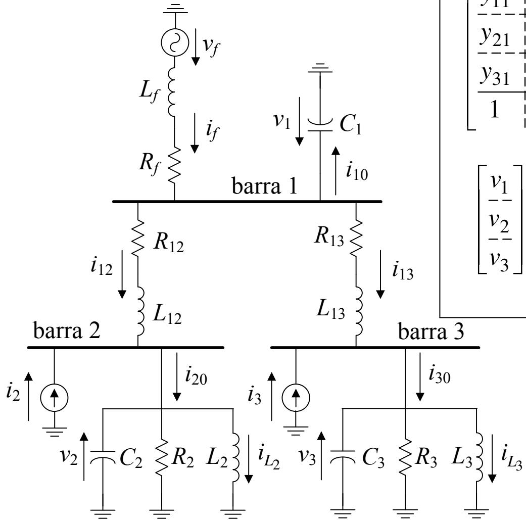
$$\left[ \begin{array}{c|c|c|c} y_{11} & y_{12} & y_{13} & -1 \\ \hline y_{21} & y_{22} & 0 & 0 \\ \hline y_{31} & 0 & y_{33} & 0 \\ \hline 1 & 0 & 0 & z_f \end{array} \right] \left[ \begin{array}{c} v_1 \\ v_2 \\ v_3 \\ i_f \end{array} \right] = \left[ \begin{array}{c} 0 \\ 1 \\ 0 \\ 0 \end{array} \right] \left[ \begin{array}{c} i_2 \\ i_3 \\ v_f \\ 1 \end{array} \right]$$
