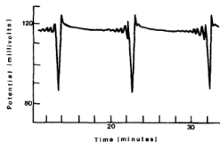
FIG. 10. Recording from bromide ion electrode; T = 25^{\circ}\text{C} ; flow rate = 5.37 ml/min; \text{Ce}^{IV} catalyst.
