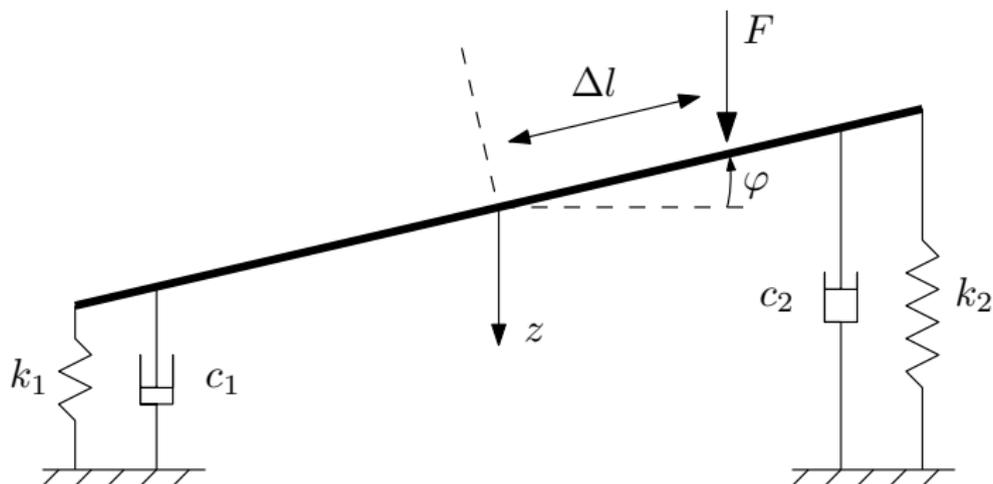
A **uniform platform** with mass  $m$  and length  $2l$ , supported in both ends by springs
