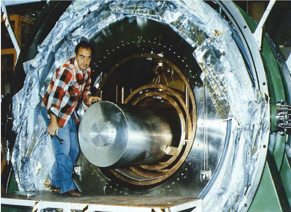
3 tonne aluminium bar, T < 100 mK, D/R in collaboration with T. Niinikoski.
