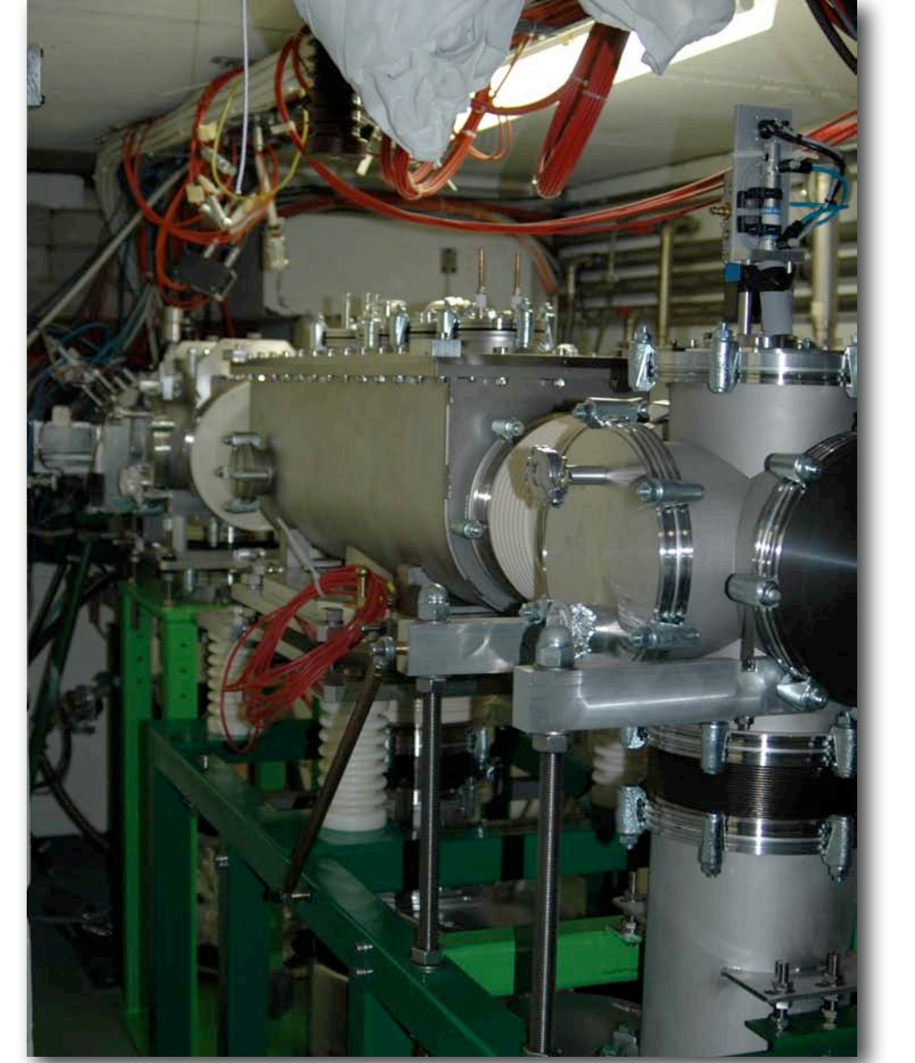
Installation of an ion-beam cooler at ISOLDE, CERN
